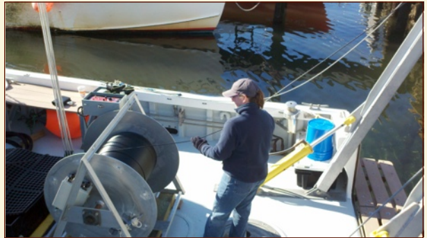
Captain Lori guiding the inductive modem wire onto the new winch. This process took approximately two hours to complete. It was important to insure the wire was spooled onto the winch neatly so as not to compromise any of the conductors.
